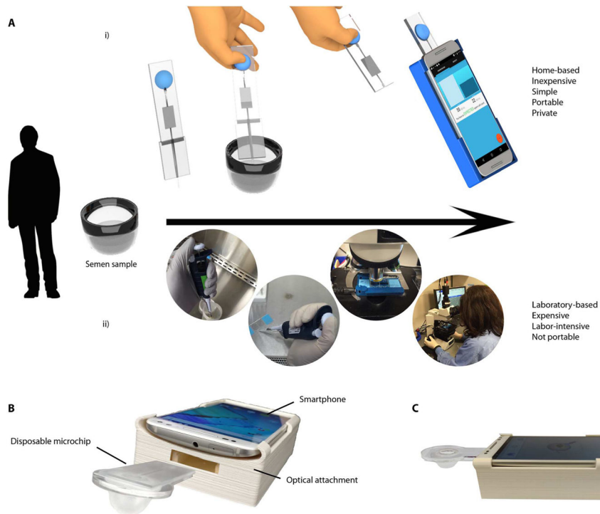
Fig. 1. The process flow for semen analysis using the smartphone-based device and conventional methods
