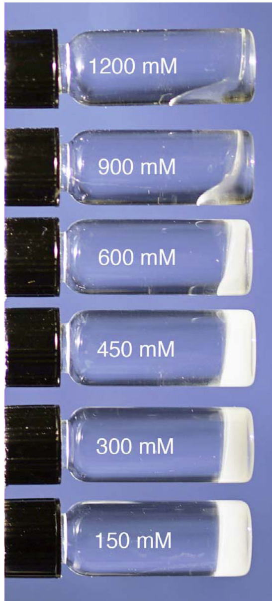
Figure 1. Morphologies of condensed Sal-IP 6 as a function of NaCl concentration. The compositions transition from liquids at high ionic strength to stiff gels at physiological ionic strength.
