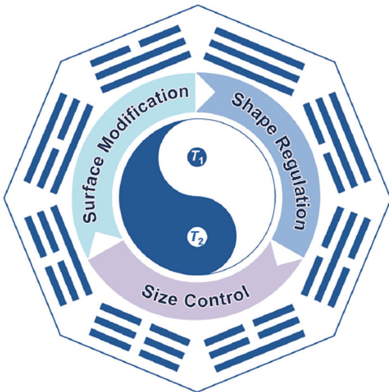
Fig. 2. Factors influencing relaxation of MRI CAs: size, surface, and shape effects at the nanoscale.
