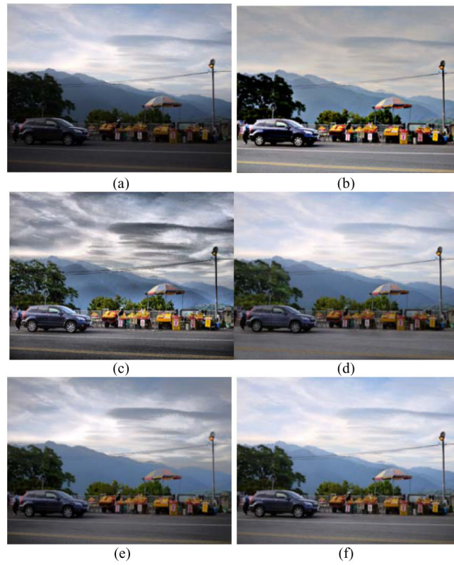
Fig. 10. Enhancement result for Lane Markers image . (a) Original image. (b) Enhanced image of MSR. (c) Enhanced image of GUM. (d) Enhanced image of NPEA. (e) Enhanced image of FHRPHS. (f) Enhanced image of NPIE-MLLS.
