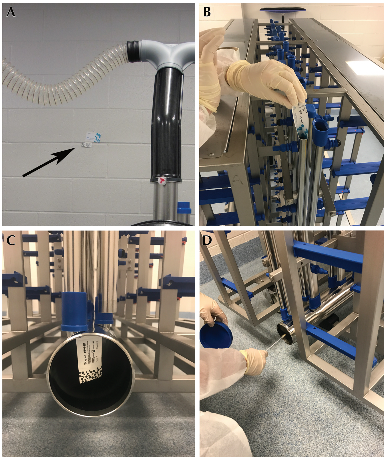
Figure 2. To assess the efficacy of each VHP cycle, indicators were placed in the room before VHP exposure, including (A) CI (arrow) on the room wall, and inside equipment airways, including (B) CI inside vertical manifolds and (C) BI inside exhaust plenums of IVC racks. In addition, specimens were collected (D) from soiled, washed, or VHP-exposed equipment surfaces and then PCR-analyzed for the presence of S. xyloso .
