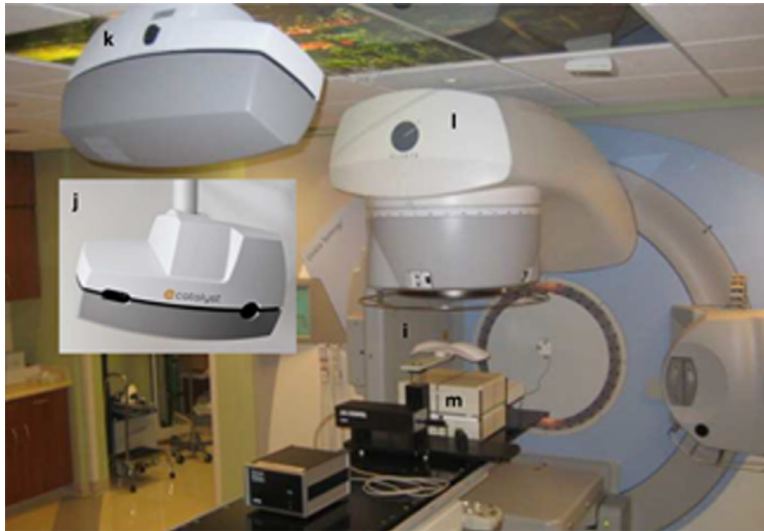
FIG. 2. Experimental setup for the gating test: i = the CIRS dynamic thorax phantom with a chest plate on the breathing platform; j and k = the front and rear views of the C-RAD Catalyst camera system; l = the Elekta Synergy linac; m = the IBA MatriXX Evolution with MultiCube and gantry angle sensor.
