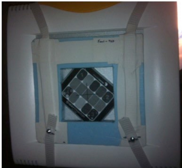
FIG. 2. The QcKv-1 phantom (note the various regions within the phantom used to assess image quality parameters) is shown affixed onto the face of one of the two flat panel detectors using an in-house jig. The jig was developed to ensure accurate centering and repositioning of the QcKv-1 phantom by indexing to the bottom corner of the flat panel detector.
