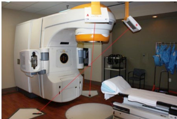
FIG. 1. The ExacTrac X-ray 6D image-guided radiotherapy system of the Novalis Tx radiation delivery system is shown. The ExacTrac system is comprised of two X-ray tubes and two flat panel detectors in the crossfire geometry.
