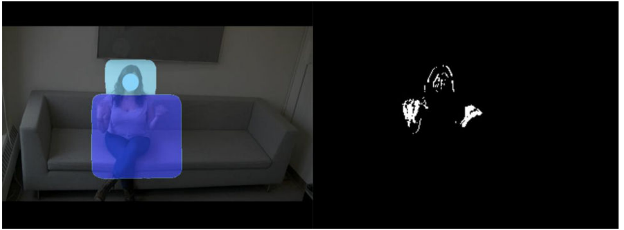
Figure 1. An example of the head and body regions of interest and the measurement of grey scale density in a movie frame. The person in the figure is a research assistant in the lab.
