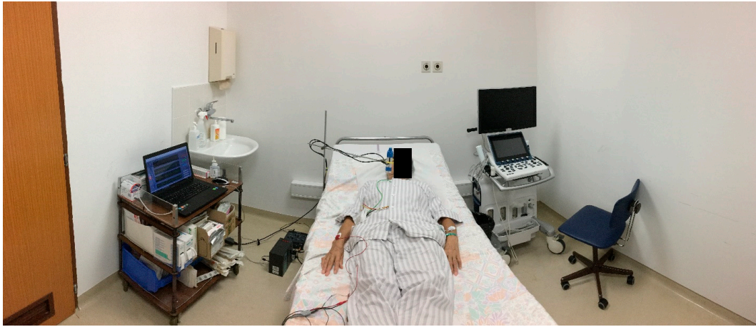
Figure 5. Clinical experiment non-contact measuring device setup.
