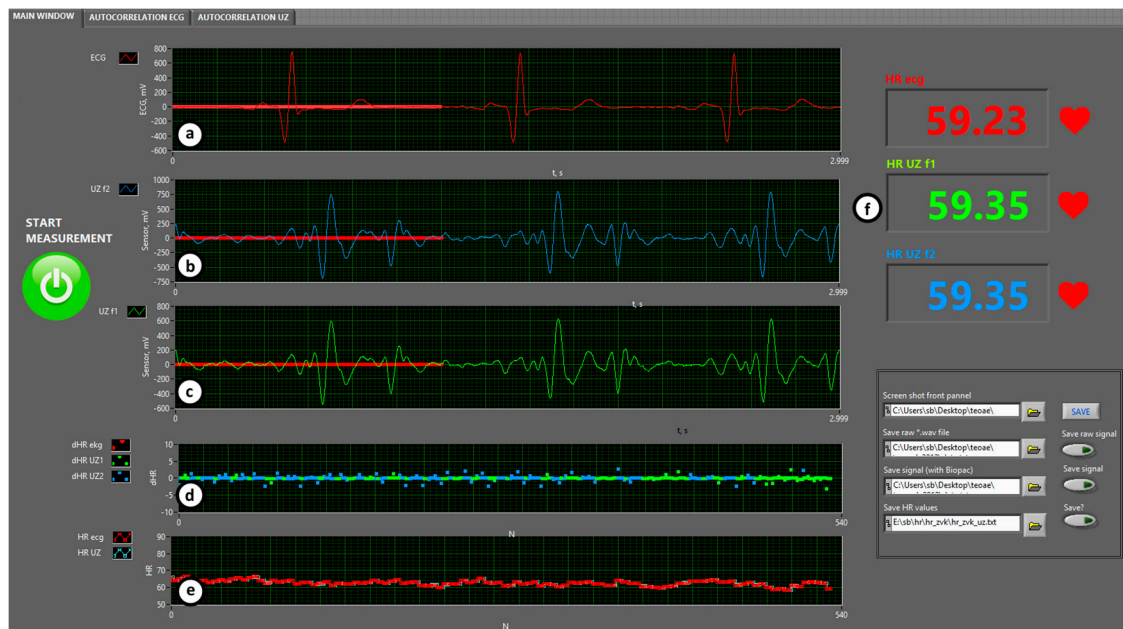
Figure 2. Front panel of the dedicated LabVIEW user interface: (a) reference III-Lead ECG signal; (b) processed ultrasound signal at f_1 = 40 kHz; (c) processed ultrasound signal at f_2 = 39 kHz. Note that US signals are delayed compared to ECG signal for about 200 ms because of the type and place of measurement; (d) measuring error, i.e., difference between the reference signal and experimental method signal instantaneous HR displayed on a diagram; (e) diagram of instantaneous HR of the two methods in question and (f) numerical display of instantaneous HR of all three signals.
