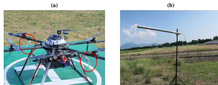
Figure 4. (a) antennas on the UAV marked as red circles; (b) the Yagi antenna at a ground station.
