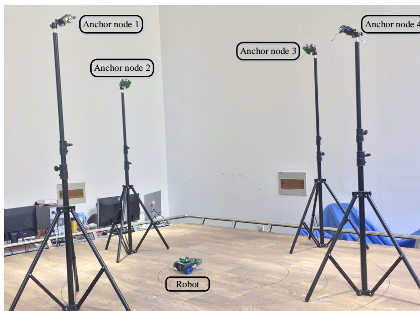
Figure 12. An illustration of the positioning experiment for the mobile robot.
