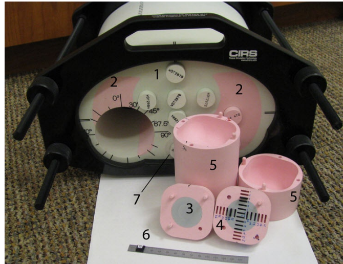
FIG. 1. An inferior view of the Thoracic Phantom: 1 – Plastic Water elliptical body; 2 – “lungs” ( \sim 0.21 g/cc); 3 and 4 – lung material dosimetric two-piece insert with the Plastic Water target and nanoDot slots; 5 – a two-piece lung cylinder accommodating the dosimetric insert in different orthogonal orientations; 6 – a nanoDot; 7 – bone density insert.
