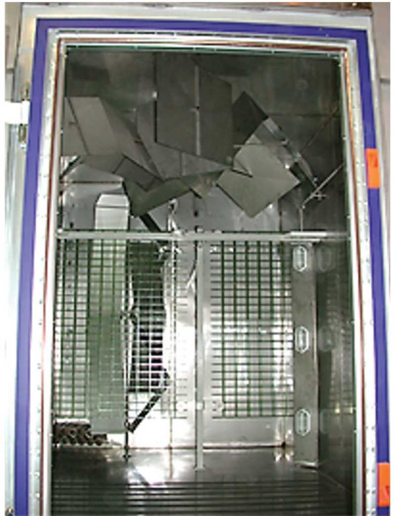
Fig. 3. Internal view of the reverberation chamber showing the two stirrers.
