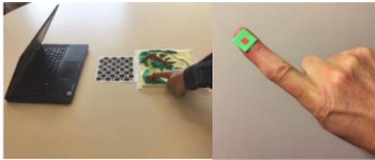
Figure 1. (a) CamIO system, showing laptop, object (relief map) and fiducial board. (b) Close-up of fingertip marker.
