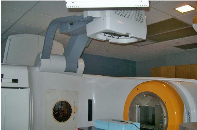
FIG. 5. The QA of beam quality and imaging dose for KV is performed with the R/F high X-ray detector placed on the top of blue styrofoam block.
