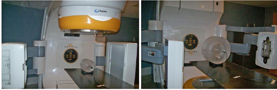
FIG. 7. The QA of imaging dose for CBCT is performed with the CTDI chamber inserted at the center hole of the cylindrical phantom.
