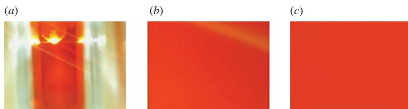
**Figure 6.** Images in various stages of processing using the OpenCV library for Python. (a) Original image ( $1024 \times 768$  pixels), (b) ROI ( $100 \times 100$  pixels) and (c) after application of  $200 \times 200$ -pixel box filter ( $100 \times 100$  pixels).
