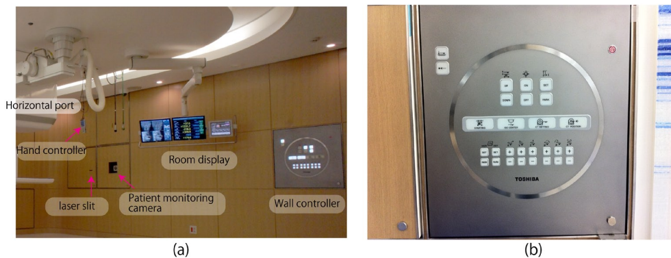
Fig. 6. Room equipment (a) including room display, hand-held/wall-mounted controllers; (b) close-up view of wall controller.
