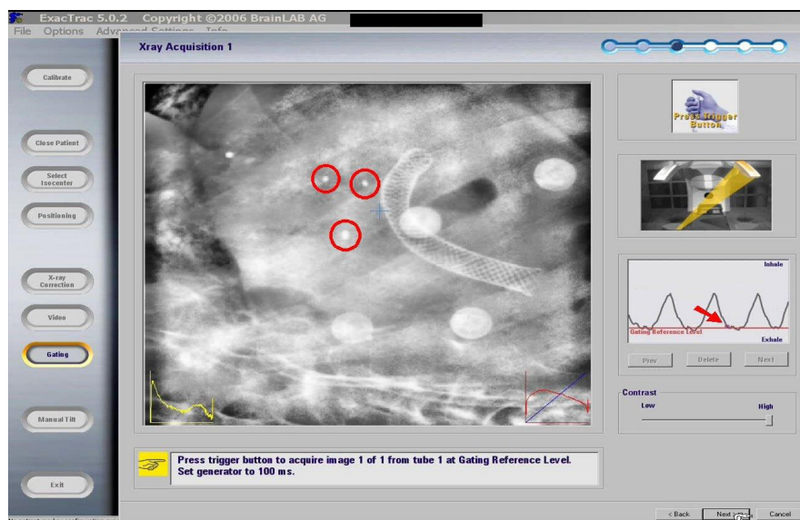
FIG. 2. One of two ExacTrac images taken at the full exhale reference level (arrow) with three fiducial markers (indicated by circles).
