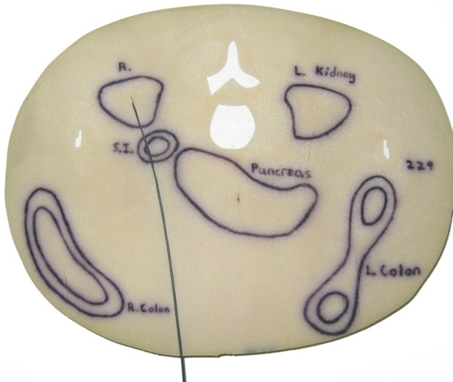
FIG. 4. Axial slice of the physical phantom with an FOC dosimeter installed in the right kidney for dose measurements (displayed in prone position but phantom was oriented in supine position for measurements).
