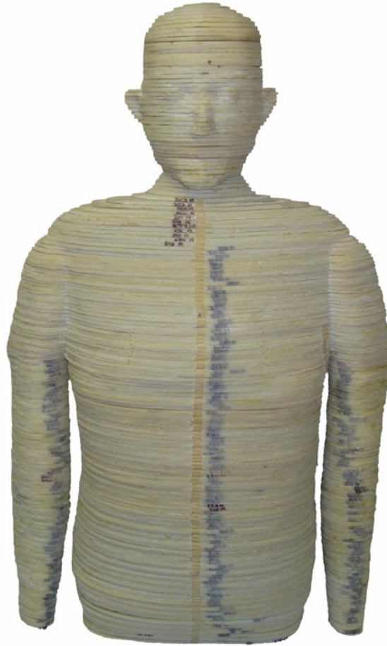
FIG. 2. Completed torso of the 50th percentile adult male anthropomorphic phantom.
