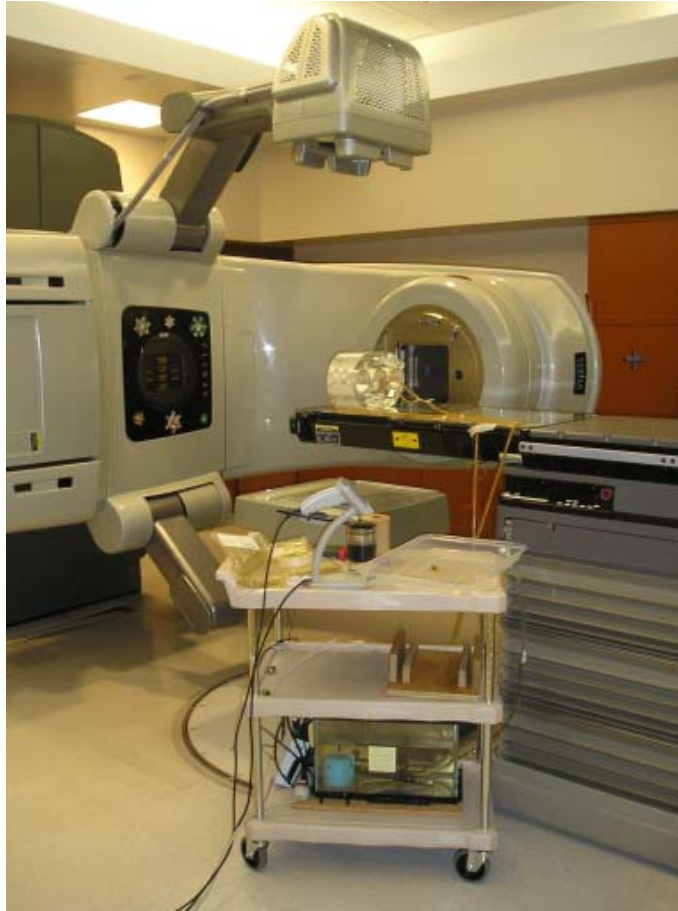
Fig. 3. Phantom setup on treatment couch and in position for kilovoltage imaging. Heated water tank is present on cart.
