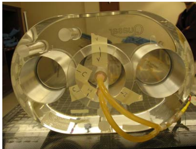
FIG. 2. Acrylic pelvic phantom with a center circular insert that can be rotated. Rubber tubing circulates heated water over the center detector (in the center of the insert) and the edge detector (at the bottom edge of the insert).
