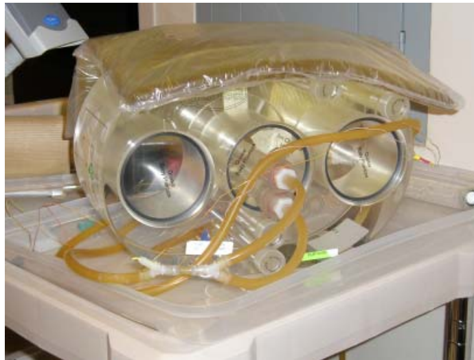
FIG. 8. Phantom with 1 cm of bolus on top. Bolus was attached with tape and could be similarly taped to the bottom of the phantom.
