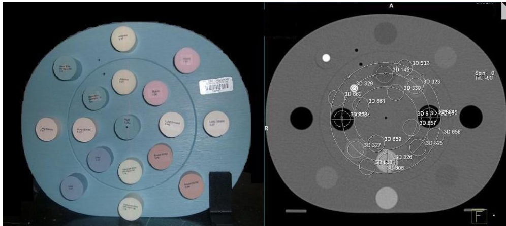
FIG. 1. Image (left) and CT (right) of the heterogeneity phantom. The regions of interests shown on the CT are the same that are used for the various CBCTs.
