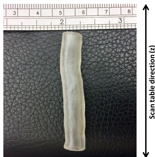
Fig. 2 Photograph of the 3-D-printed carotid phantom used in the phantom experiments. The basic model was generated using CT angiographic images from a patient. The lumen is \sim 5 -mm in diameter, and the wall is \sim 2 -mm thick.
