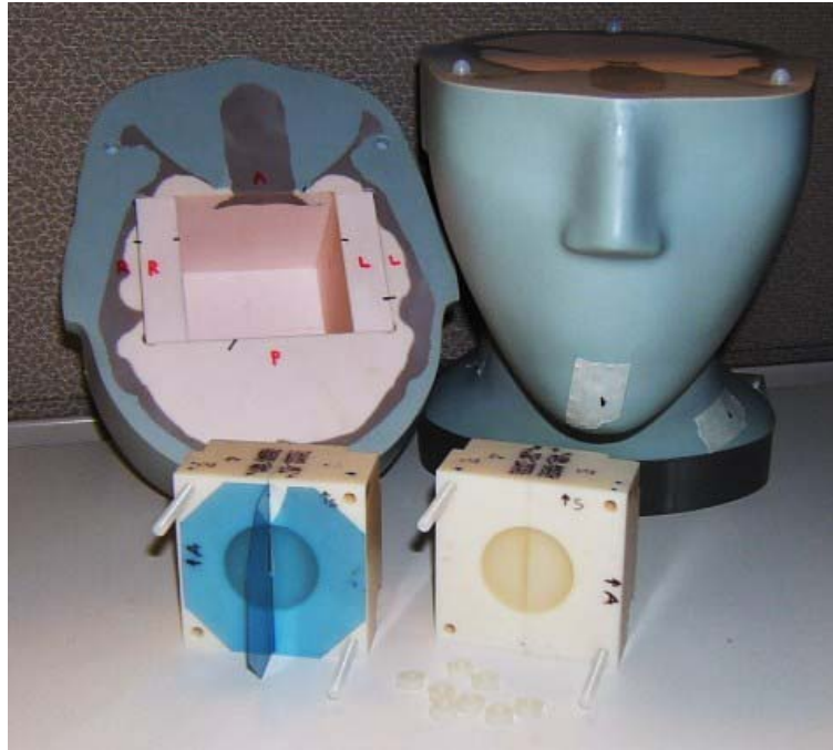
FIG. 1. Disassembled ball-cube phantom used for the global hidden target test.
