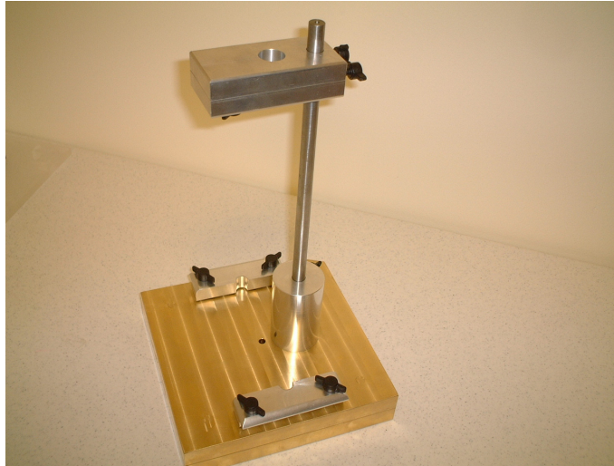
FIG. 1. Mechanical jig used for testing the gantry isocenter alignment at the Proton Therapy Center in Houston. The base is a brass plate (4-cm thickness) that supports the film holder on a 30-cm metal rod. The brass plate has a central hole (8-mm diameter), and the film holder has a corresponding hole (20-mm diameter). This mechanical jig is loaded in the snout.
