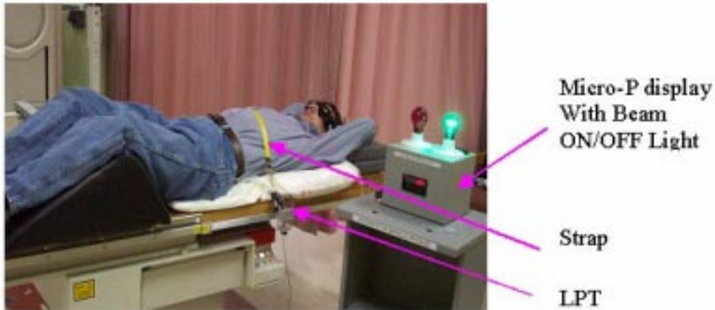
FIG. 2 Patient setup showing the strap around the patient's chest and the LPT attached to the railing of the bed
