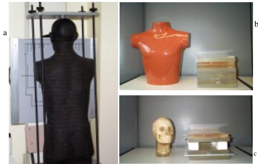
FIG. 1. The five anthropomorphic and physical phantoms used in this study: (a) Alderson Rando; (b) chest RSD-77SPL and uniform; (c) skull 3M and AAPM31.
