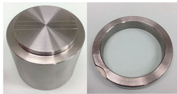
Figure 1. Block test and ring mold made according to ISO 4823:2000.
