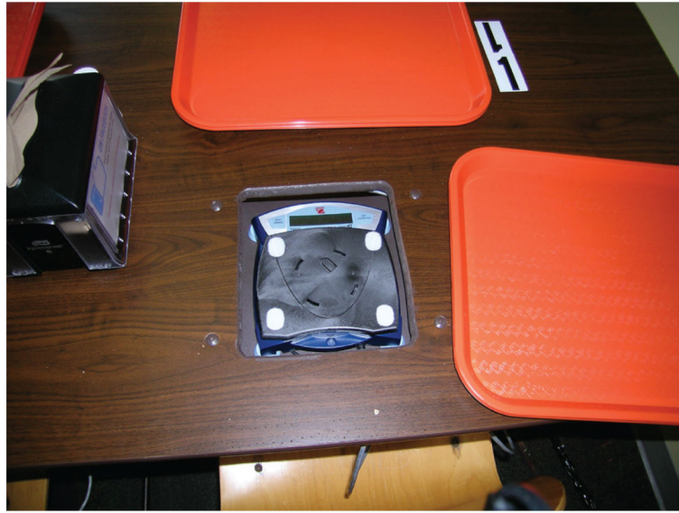
Fig. 5. A scale was mounted beneath each participant's tray.
