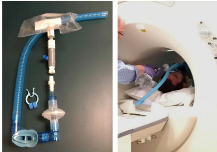
Figure 12. Components of a dedicated system for HP gas delivery to imaging subject (left) and view of the system in use (right). The bag containing HP gas is attached to the breathing apparatus just prior to inhalation and imaging. Unidirectional valves ensure inhaled gas is only drawn from the HP gas bag, while exhaled gas exits through flexible tubing and is vented outside of the scanner bore. Image adapted from [305].
