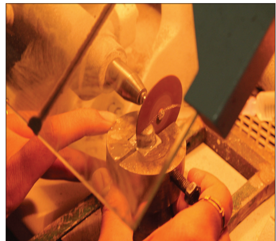
Figure 9: Sectioning of samples
