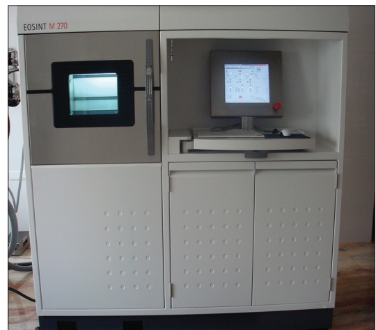
Figure 7: Direct metal laser sintering machine (EOSINT M270, EOS GmbH, Germany)
