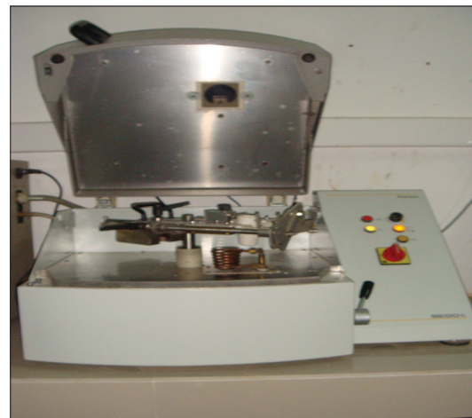
Figure 5: Casting machine (Bego, Bremen, Fornex T)
