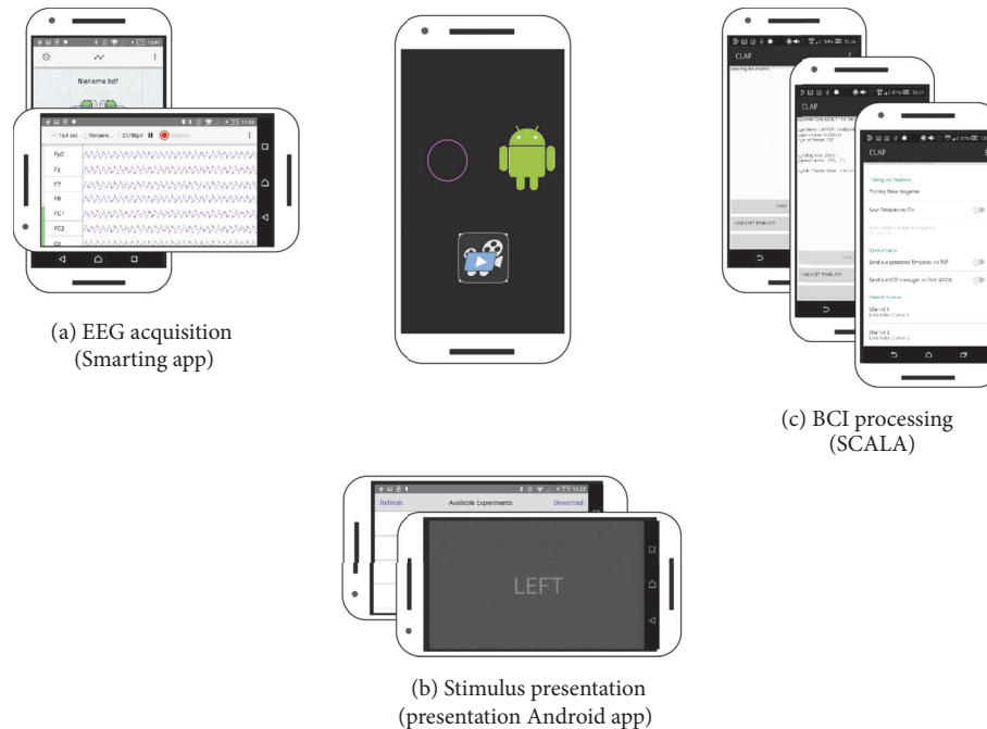
FIGURE 1: The multiapp BCI on Android approach. An EEG data acquisition application (a) and a stimulus presentation application (b) communicate with our BCI signal processing application SCALA (c). All three applications run on the smartphone during an experiment. They exchange data using socket-based, synchronized communication.
