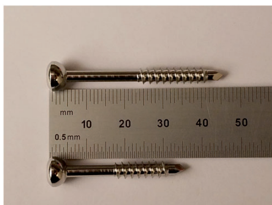
Figure 4. Photograph of the Synthes 4.5 mm steel Large Fragment LCP System malleolar screw.
