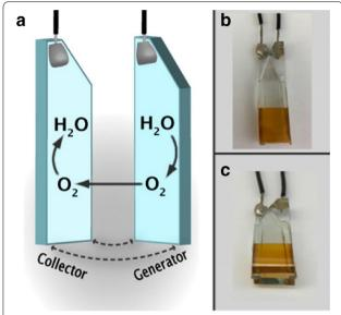
**Fig. 7** a Collector–generator schematic and photographs of the front (**b**) and bottom (**c**) of an example C–G assembly consisting of a FTO|nanoTiO<sub>2</sub> photoanode derivatized with a chromophore–catalyst assembly and a FTO collector electrode (Reproduced with permission from ref [49]. Copyright 2016 American Chemical Society)
