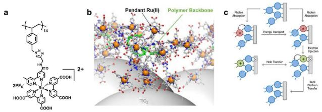
**Fig. 4** a Structure of carboxylic acid-derivatized polymer, **PS-Ru-A**. **b** Cartoon of PS-Ru-A anchored to a TiO<sub>2</sub> nanoparticle surface. **c** Schematic representation of the photophysical events of the PS-Ru-A assembly at the surface of TiO<sub>2</sub>. The blue circles represent Ru(L)32 + chromophores while the green and red circles correspond to Ru(L) $_3^{3+}$  and Ru(L) $_3^{2+*}$  (Reproduced with permission from Ref. [18]. Copyright 2016, Wiley–VCH Verlag Gmbh & Co)
