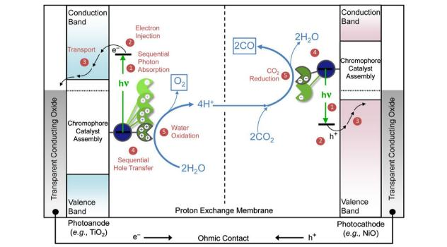
Fig. 1 Schematic diagram for a tandem DSPEC for solar-driven  $CO_2$  splitting into CO and  $O_2$  by the net reaction,  $2CO_2 + 4 \text{ hv} \rightarrow 2CO + O_2$  (Reproduced with permission from Ref. [5]. Copyright 2016 American Chemical Society)
