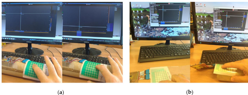
Figure 12. (a) Performance test on a curved surface touching two different points; and (b) performance test touching on the same point but on a flat and a curved surface, obtaining the same result.
