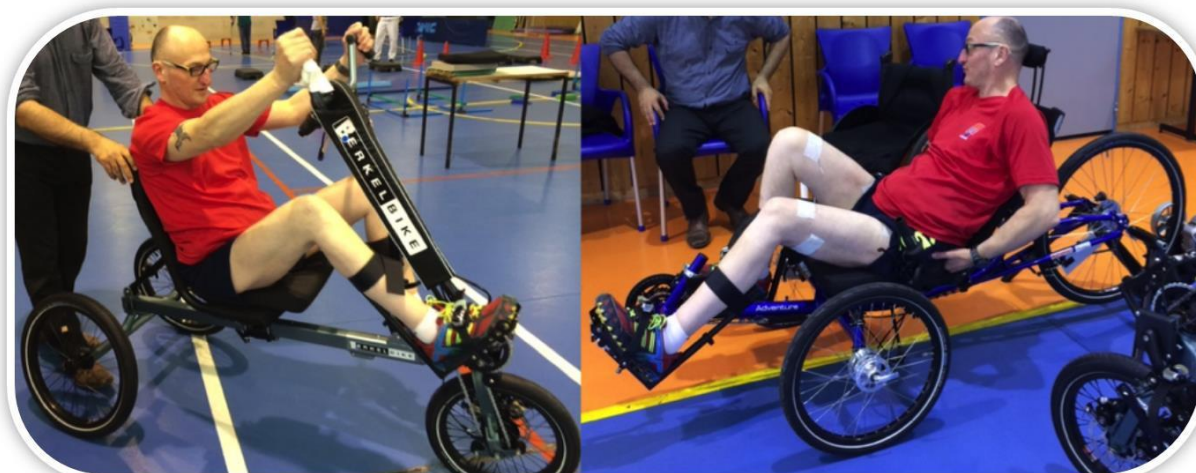
Fig 1. The two trikes used (left) during the initial training program, the Berkelbike Pro® and (right) for the final training program and at the competition, the FreeWheels trike
