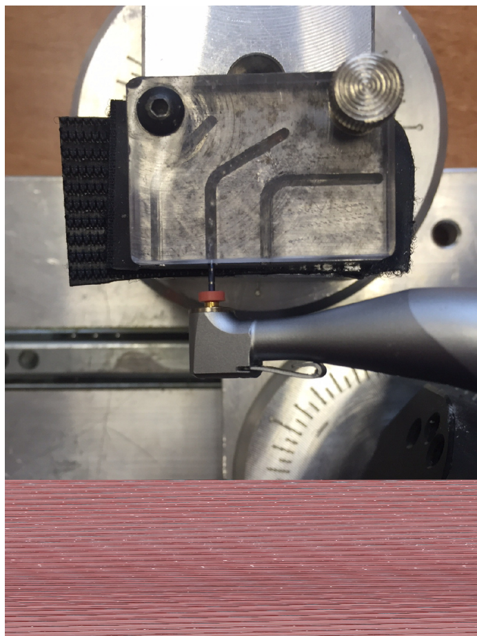
Figure 1. The testing device for cyclic fatigue.
