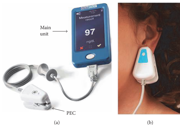
FIGURE 2: GlucoTrack NI monitoring device. (a) The device includes a main unit and three different sensor pairs, one per each of the three technologies, and all located at the tip of a personal ear clip (PEC). (b) Illustration of glucose measurement performance using GlucoTrack. The PEC is clipped to the earlobe for spot measurement.
