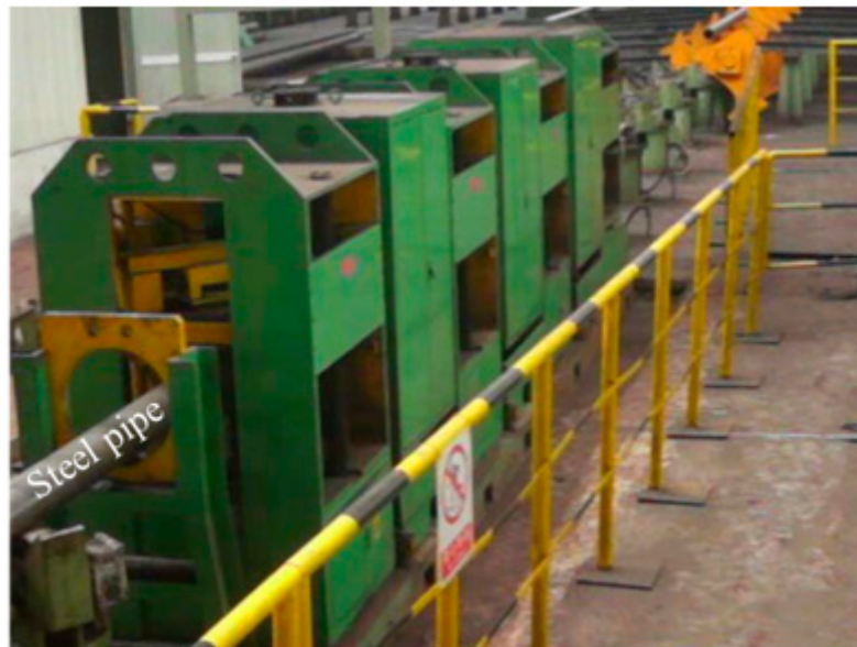
Figure 11. The whole online MFL inspection apparatus for steel pipe.
