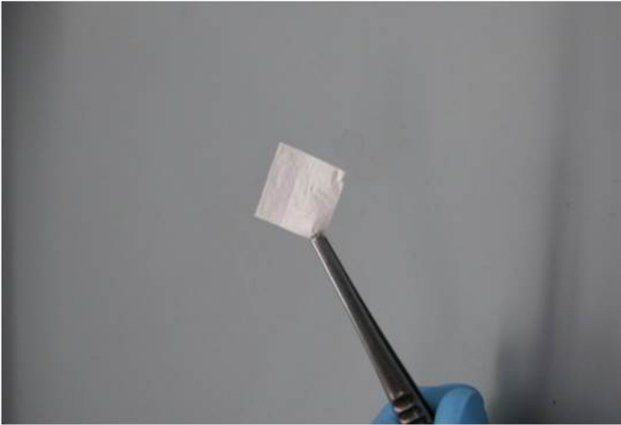
Figure 1: 2 x 2 cm Section of SIS Used for Repair of Experimental Ventral Abdominal Hernia. The SIS material is an acellular extracellular matrix derived from porcine small intestinal submucosa. Please click here to view a larger version of this figure.
