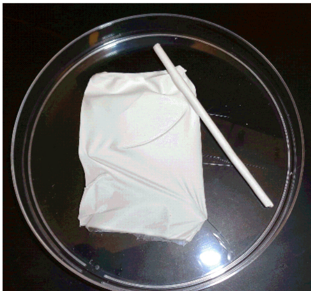
Figure 1: The macroscale morphology of electrospun fibers. The electrospun fibers shown were fabricated using a 4 mm (cylinder) and 25 mm (sheet) diameter mandrel, respectively. Please click here to view a larger version of this figure.
