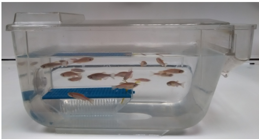
Figure 3: Breeding device submerged in a fish holding tank to collect sludge for analysis. This tank is set on a bench for the purpose of the picture; it is set otherwise in the recirculating system. Please click here to view a larger version of this figure.
