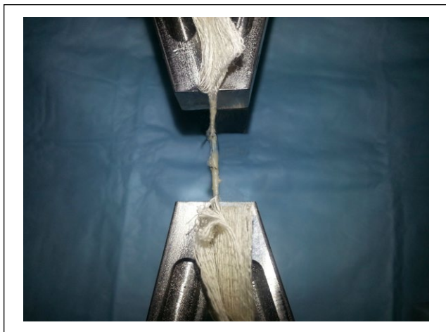
Figure 4. Picture of a nerve placed in the tensile testing machine.
