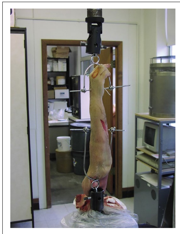
Figure 1. Cadaver specimen attached to Instron device for application of axial loads.
