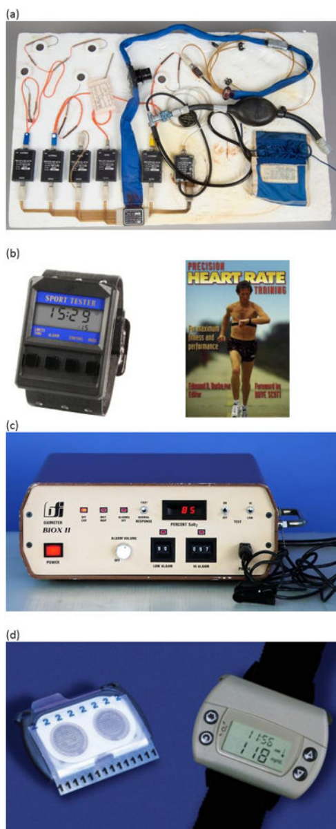
Figure 1. Historical examples of sensors including (a) wearable sensors for the Apollo Space Program 2 , (b) Polar's 'Sport Tester PE2000' heart rate monitor, (c) pulse oximetry worn on the fingertip, and (d) non-invasive chemical glucose sensing with the GlucoWatch product 3 (discontinued). The devices shown in (a) and the pulse-ox meter in (c) were wearable, but they were not wireless like the devices shown in (b) and (d).
