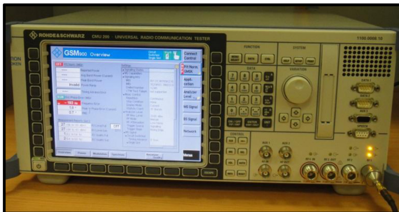
Fig. 1. CMU 200 generator used to generate the frequencies of electromagnetic radiation.
