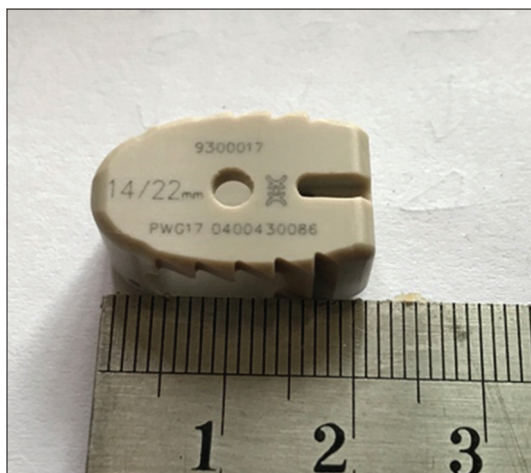
Figure 2: The polyetheretherketone cage used in our study.
