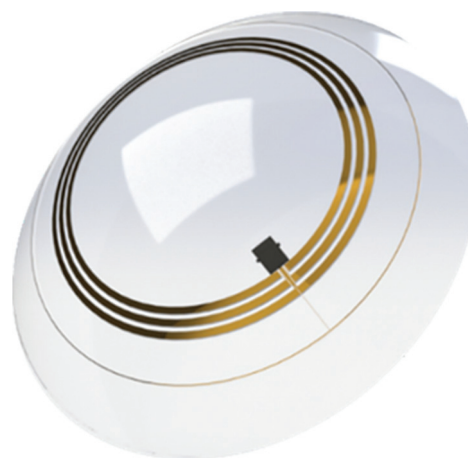
Figure 3. Diagram of a contact lens IOP sensor that includes a strain gauge sensor placed circumferentially, an antenna for telemetry and wireless powering, and a microprocessor. IOP, intraocular pressure
