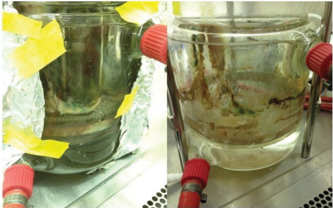
Figure 4. Biofilm build up in the bioreactor vessel during evolution of P. aeruginosa to colistin The bioreactor design favors the development of strong biofilms. Since the evolution of the populations takes place over weeks in a single vessel, those adaptive alleles that favor biofilm formation have a selective advantage as they can adhere to surfaces and not be removed as new media is added to maintain a constant exponentially growing planktonic phase. Acinetobacter , enterococci, and Pseudomonas have all exhibited strong biofilm formation in this experimental system.
