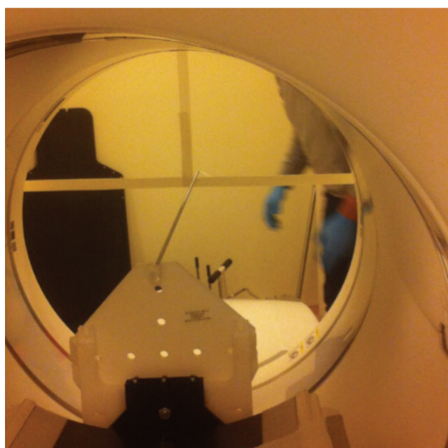
Figure 2. National Electrical Manufacturers Association sensitivity phantom on the (up), centering the source on the (right)
