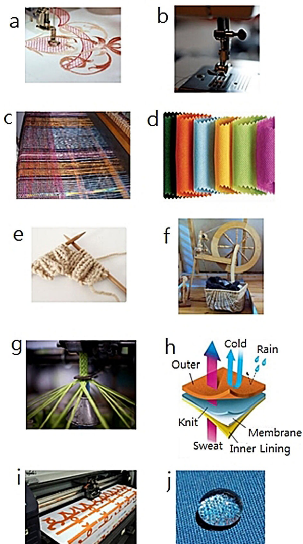
Figure 13. Different kinds of textile/fabric manufacturing. a) Embroidery, b) sewing, c) weaving, d) nonwoven, e) knitting, f) spinning, g) braiding, h) coating/laminating, i) printing, and j) chemical treatment. Reproduced from Ref. [55] with permission of MDPI.
