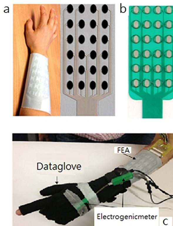
Figure 6. a) Fabric electrode array. b) Flexible printed circuit board (PCB) array from Fatronik–Tecnalia. c) Monitoring system for a fabric electrode array (FEA) based on hand movements. Reproduced from Ref. [39] with permission of Elsevier.
